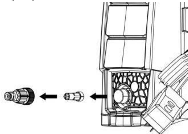
Clean the nozzle with the needle clean-out tool provided . Remove the spray
