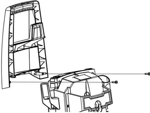
**2. Slide the trigger gun holder into position of unit left .**
