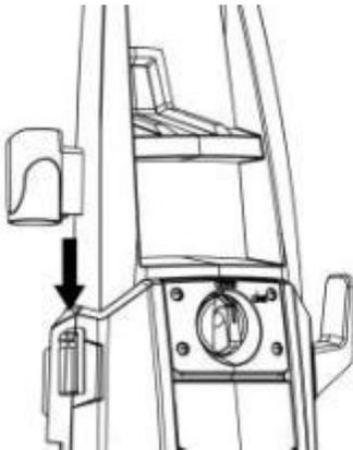
**3. Installing the power cord hook into position of unit right**
