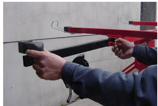
Fig 10. To extend the outriggers for use, pull out on the outrigger lock pin with your right hand and slide the outrigger out with your left hand as shown. The lock pin will engage at different points on the outrigger. MAKE SURE that the lock pins are engaged in one of these positions before loading the unit. Retract the outriggers when storing or transporting the unit.
