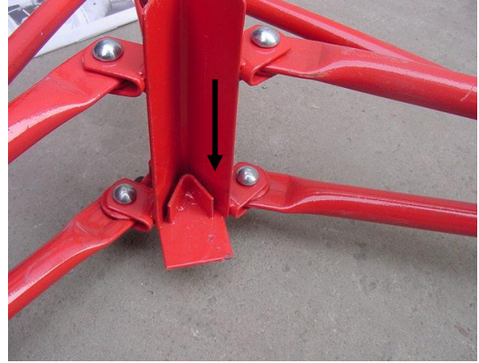
Fig 2. To hold the tripod base in position during this procedure set the backstop as shown.
