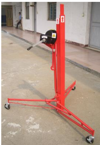
Fig 5. When the frame is correctly positioned on the tripod base release the backstop.
