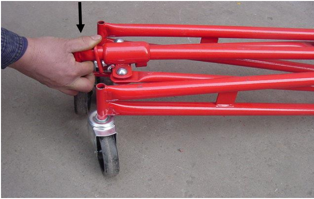
Fig 1. Begin by setting up the tripod base: press down on the slide yoke ring and swing the outer legs out until they lock in the working position (note the holes on the bottom of the slide tube).
