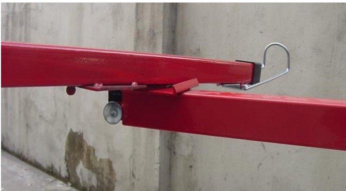
Fig 9. Place the tapered plates of the crossarms into the tapered sockets on the cradle. The spring tab on the back of the crossarm will lock it into place.
