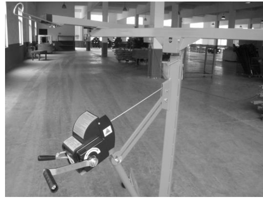
Fig 8. Mount the cradle on top of the telescoping section. Flip out the tilt latch to allow the cradle to tilt for loading and for hanging drywall on sidewalls and sloped ceilings.
