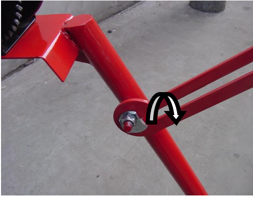
Fig 7. Make sure that the safety plate in the socket of the slide bar.
